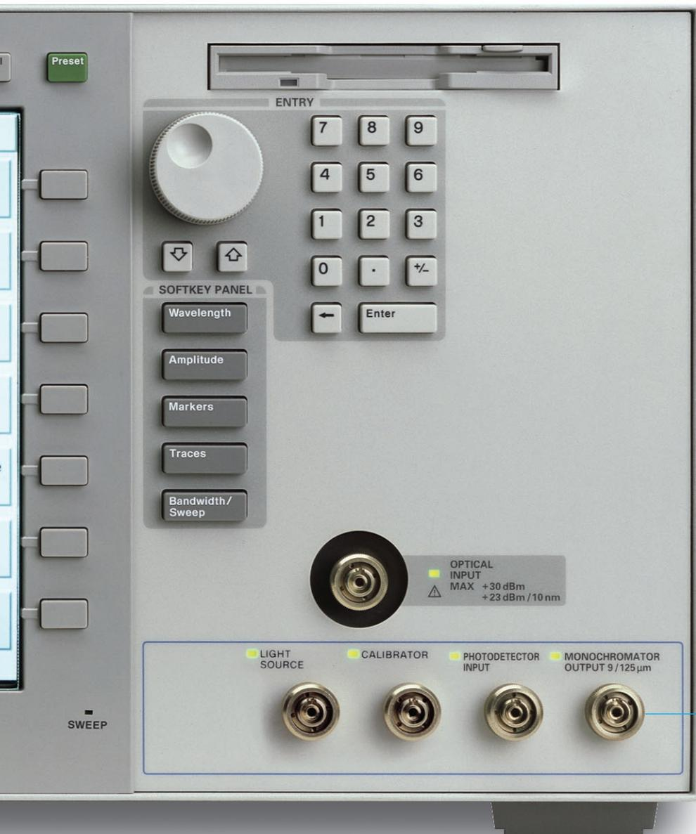
**The Internal EELED** broadband light source is ideal for passive component test and reduces the number of instruments required to perform passive component measurements.
