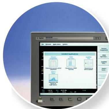
The 86146B OSA also has a built in Time Domain Extinction (TDE) method for measuring amplifiers. TDE can very accurately measure ASE power of amplifiers with slow relaxation states, such as Erbium Doped Fiber Amplifiers (EDFAs) and Erbium Doped Waveguide Amplifiers (EDWAs).
